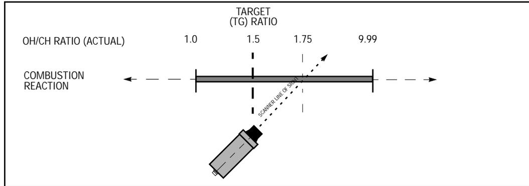
The changes in the OH/CH ratio is sensed by the scanner and transmitted to the controller. The controller compares the actual OH/CH ratio to the TARGET RATIO (TG) for that specific firing rate. (Refer to the **LEARN OPERATION** under the **LEARN GROUP** section of this bulletin.). When the controller sees a difference between the TG and the actual OH/CH ratio, it generates an output to the CA202 trimming actuator to reposition the burner air damper.
