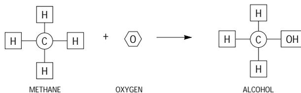
Or, methane plus oxygen equals an alcohol. The collision force actually drives the oxygen atom into a methane molecule. The opening of the chemical linkages holding the atoms releases the energy of these linkages, raising the temperature of the molecule. The second phase is:
