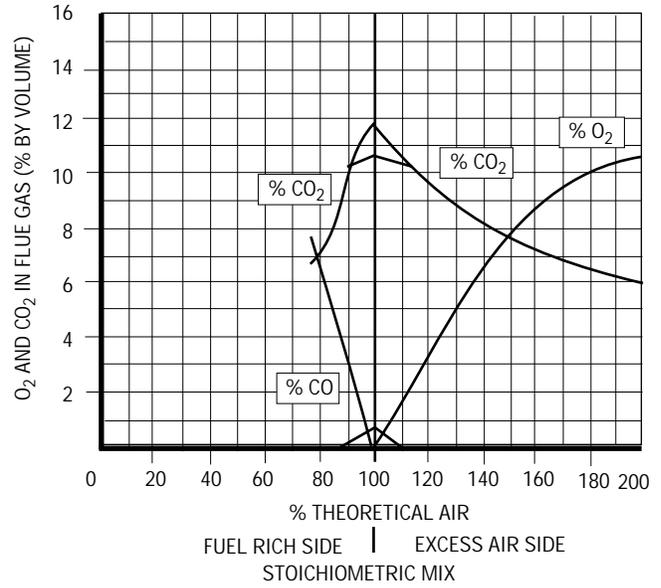
CONVERTING BETWEEN WET % O<sub>2</sub>, DRY % O<sub>x</sub>, AND % EXCESS AIR
