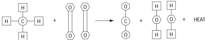
At about 1200°F enough velocity and energy has been imparted to molecules so that the collision occurs with enough force to break the double oxygen bond and hydrogen linking to the carbon center of the methane molecule. At this time, the situation is very unstable. The carbon has a high affinity for oxygen and so does hydrogen. Combustion begins.
