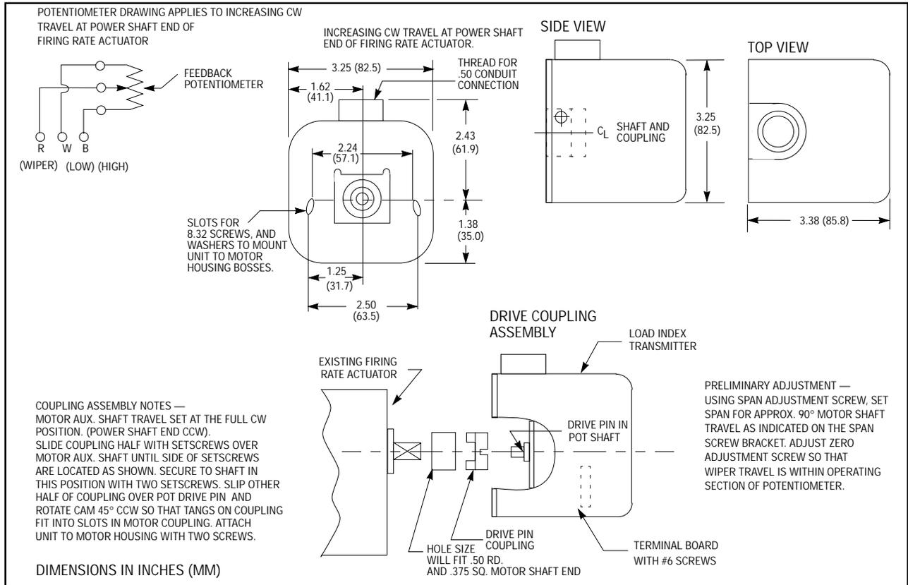
**FIGURE 5. TYPICAL FIRING RATE FEEDBACK POTENTIOMETER TRAVEL (90° MINIMUM)**
