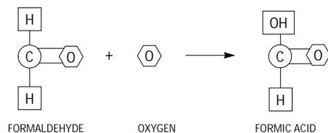
The step-by-step reaction is proceeding with increasing releases of energy and a constantly rising temperature level. In this high-energy state, formic acid is unstable and breaks down with the oxygen to form carbon monoxide and the second water molecule is released.
