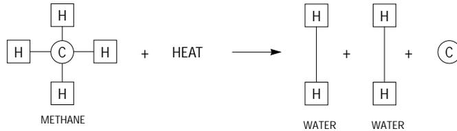
At these temperatures the carbon atoms are incandescent and they impart a yellow glow to the flame. Some luminous flame nozzle mixing burners deliberately control the rate of air addition to moving gas stream to produce maximum flame color.
