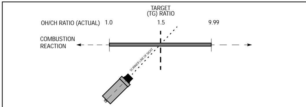
In Figure 11, Target Ratio (TG) of the combustion reaction has moved to the right causing the scanner to view a lower ratio. This shift was caused by the fuel/air ratio becoming richer. To correct for this change in fuel/air ratio, the trimming actuator needs to open the air damper, increasing the air supply. This increase in air causes the combustion reaction to move left, repositioning the original OH/CH TARGET RATIO (TG) in front of the scanner.
